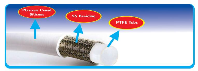
**RekTef** is PTFE tubing covered with SS 304 braid reinforcement having outer layer of Platinum grade silicone. **RekTef** is having capacity to withstand high pressure along with greater chemical resistance. The product is having ultra smooth bore which enhances superior flow properties & least adhesion to particulate. The outer layer of Silicone cover acts as insulation to high temperature and keeps outer surfaces dust free.
